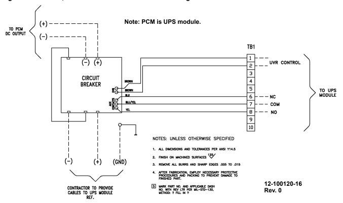
Figure 124 48 UVR, circuit breaker to terminal block wiring
